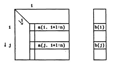
In the k-th step of backsolving the triangular system, the trailing part of the k-th row of A is multiplied by the computed part of the solution vector x as shown below:
