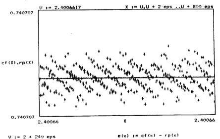
The next graph shows how roundoff obscures rp(x), but not cf(x), by about 24 times as much as that function
