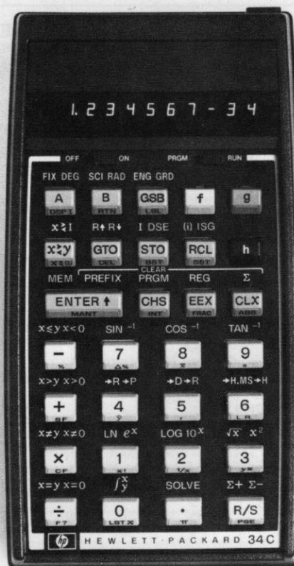
Fig. 1. The HP-34C, a new handheld programmable calculator, has two keys that are new to handheld calculators— \int (integrate) and SOLVE , a numerical equation solver, is described in this article.
